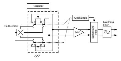
Figure 3. Concept of Chopper Stabilization Technique
