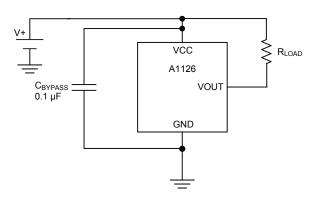
Figure 2. Typical Application Circuit
